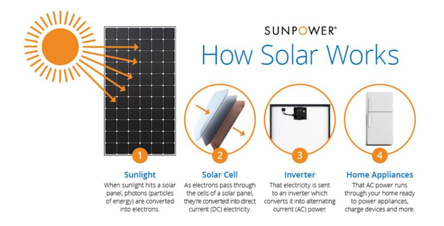
When sunlight shines on the solar panels, it generates DC (Direct Current) power. Inverters change the DC into AC (Alternating Current) power. Solar panels will provide power to your home first.
